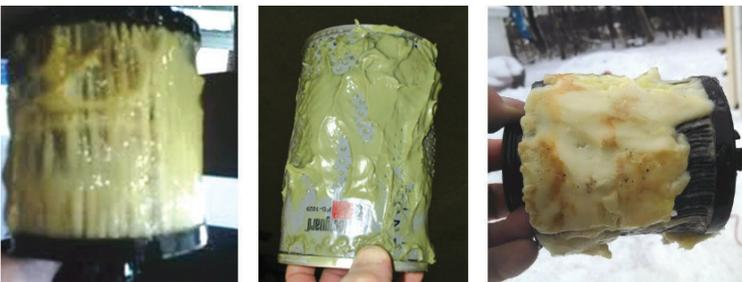
As fuel temperatures decline, waxes in diesel fuel can coagulate - forming crystals that block fuel lines and filters.
